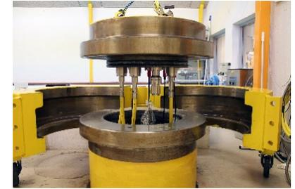
Hydrostatic pressure testing
